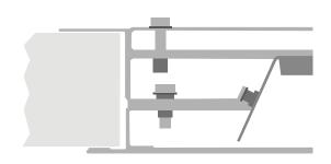
NOTE: The Evo RA XL integrates in to the ceiling panel to maintain the working platform in the void space.
