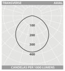
Luminaire Lumen Output 35W = 3120lm 72W = 6240lm
