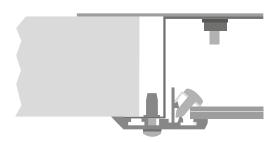
NOTE: The Zeta FA integrates into the ceiling panel to maintain the working platform in the void space.
