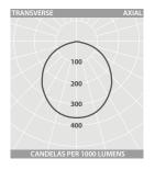
LED LED Luminaire Lumen Output 26W = 4137lm 35W = 5570lm 47W = 7480lm 54W = 8594lm 70W = 10617lm 84W = 12740lm 84W = 12740lm Emergency = 509lm\*
