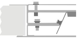
NOTE: The Evo RA integrates in to the ceiling panel to maintain the working platform in the void space.
